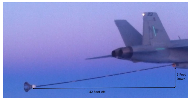
FIGURE 5 F/A-18 Equipped with an ARS pod streaming a drogue behind it with Approximate dimensions labeled 34
