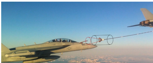
FIGURE 4 EA-18G Growler at the pre-contact position with a proposed clearance envelope superimposed on the image 33
