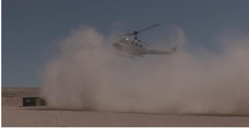
Fig. 11 System under test performing an autonomous landing during full brownout conditions at Twentynine Palms Marine Base during flight 59F120 [89].
