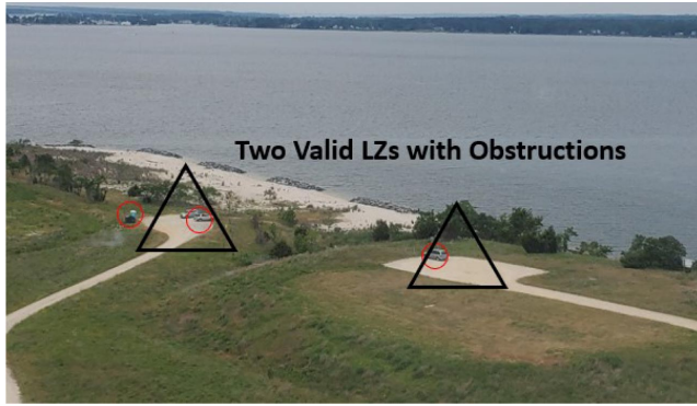
Fig. 4 Pilot's perspective of two LZs that would have been valid if the vehicles were not present, taken from a UH-1 at 200 ft AGL over the turf training area of NAS Patuxent River [95].
